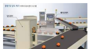
4. Inspection of weight and internal quality
