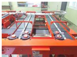
Discharge Standby Conveyor
